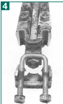
4 Flourocarbon and Moly DiSulfide coatings too easily penetrated
