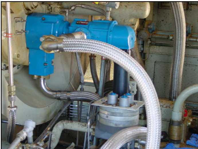
Figure 7. Air Starter Installation
