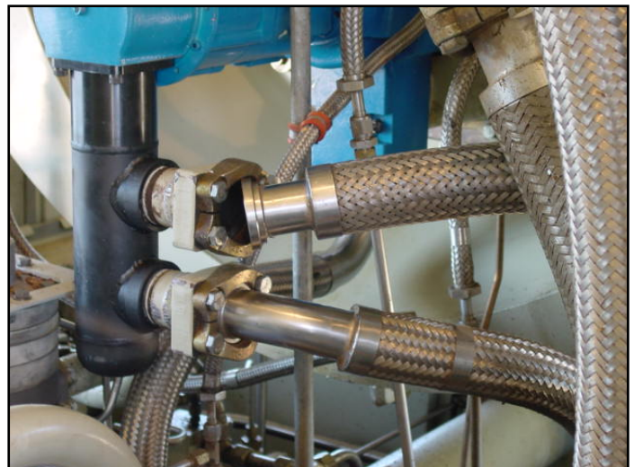
Figure 8. Exhaust Hose Installation
